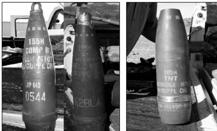
Figure 9: 155mm Composition B shell, 155mm TNT shell, and 105mm TNT shell (left to right) detonated during the Bronze Scorpio field tests.
