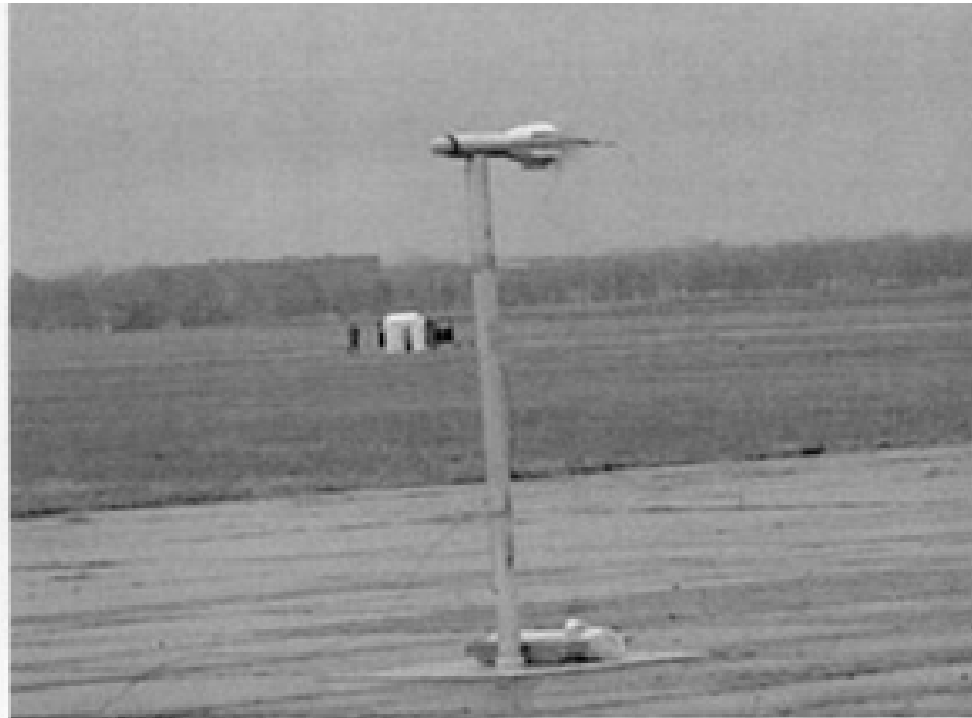
Figure 11: Dual Thrust Smokey SAM test setup at Wright Patterson AFB, Area B Test Range. The DTSS was fixed approximately 1.5 meters above a concrete runway.
